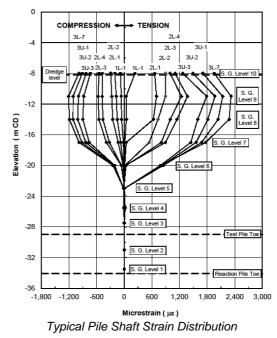
Strain gauges cast into the concrete during pile construction were monitored to provide strain measurements along the pile shaft. This data was used for the calculation of bending moment profiles and as a prediction of lateral deflection which compared favourably to deflection profiles taken from cast-in inclinometer tubes. However, strain gauge data should always be considered as a backup secondary means of determining lateral deflection and bending moment profiles.
