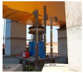
Arrangement of Jack and Load Cells
