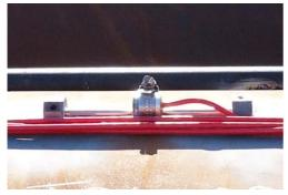
Strain Gauges Fixed To Test Piles
