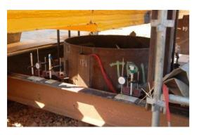
Typical Setup of Displacement Gauges
