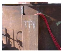
Strain Gauge Protection Channel
