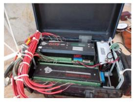
Strain Gauge Leads Connected To Data Logger
